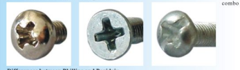
Differences between Phillips and Pozidriv Pozidriv is similar to Phillips but designed not to slip, or cam out. It does not have the rounded corners that the Phillips screw driver has. Phillips screwdrivers will usually work in Pozidriv screws, but Pozidriv screwdrivers are likely to slip or tear out the screw head when used in Phillips screws. Pozidriv heads are marked with crossed, single lines at 45 degrees to the cross recess, for identification. JPCI should only use Pozidriv and not Phillips
