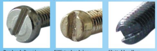
Pan head: Provides a low large diameter head Filler head: has a smaller diameter than the pan head, but is higher with a correspondingly deeper slot. Used in connection blocks Slotted headless: This type of screw is used as a calibration screw inside thermostats or controls shafts
