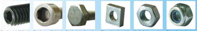
Hexagonal socket headless: Has a hexagonal hole and is driven by a hex wrench. Hexagonal socket: Has a hexagonal hole and is driven by a hex wrench. Hexagon head: Standard type of wrench-applied hexagon head. It has sharp corners trimmed to close tolerances. Square: This nut is used inserted in plastic parts Hexagonal: Standard nut Nylon top: This nut has a nylon ring that avoid unscrewing by vibration
